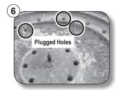
EXAMPLE: Close-up of a Generator with excessive scale deposits. The holes are plugged and should be cleaned according to Owner's Manual 1010699.
