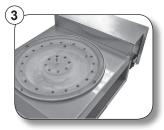
Inspect <u>all</u> 26 generator holes and the two side water injection holes. They should NOT be plugged.
